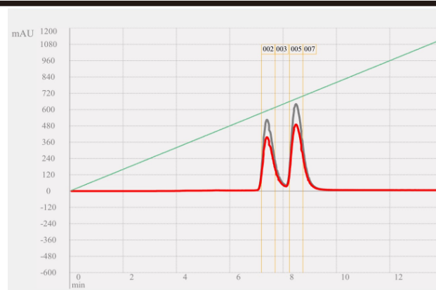
Figure 3. The separation of A and B by SepaFlash® HP Platinum (Spherical, 20 - 45 \mu\text{m} , 70 \text{\AA} , SW-2102-040-SP)
