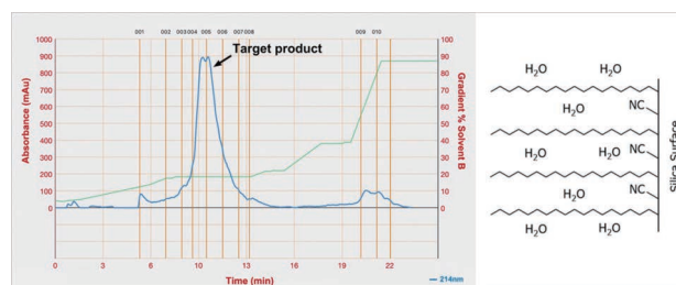
Figure 3. The flash chromatogram of the sample on a C18AQ cartridge.
