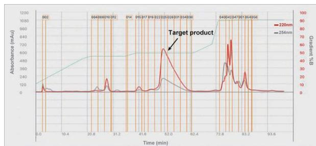
**Figure 6.** The flash chromatogram of the synthetic product on a 120 g flash cartridge.
