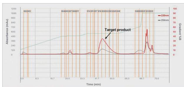
**Figure 5.** The flash chromatogram of the synthetic product on a 25 g flash cartridge.
