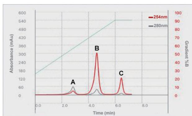
**Figure 3.** The flash chromatogram of 4.0 mL sample mixture on an 80 g flash cartridge.
