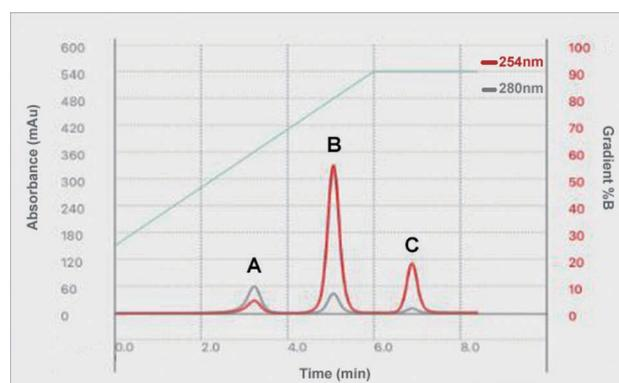
**Figure 2.** The flash chromatogram of 1.2 mL sample mixture on a 25 g flash cartridge.
