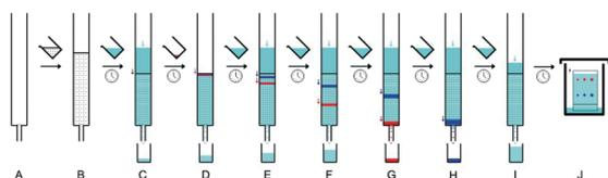
**Figure 1. Schematic diagram of traditional manual column chromatography. A–B: Column packing. C: Column equilibrium. D: Sample loading. E–F: Elution. G–H: Fraction collection. I: Column cleaning. J: Detection by TLC.**
