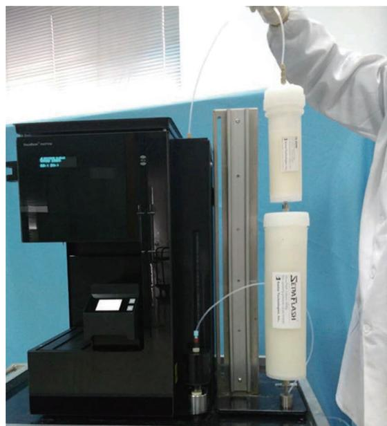
**Figure 3. The experimental setup for automatic flash chromatography.**
