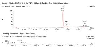
Conclusion, excellent separation of CBD and THC can be achieved with Santai Spherical reverse-phase C18 silica column. Since C18 columns are reusable at least 30 times with proper storage, this is an effective and economical method for the isolation of CBD and THC.
