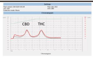
As demonstrated here, our SepaBean™, automatic flash chromatography system is an excellent and efficient instrumental tool to purify CBD from Cannabis. It is equally effective for the purification of THC. This flash chromatography method is a simple, rapid and effective method for the isolation of key compounds in Cannabis.
